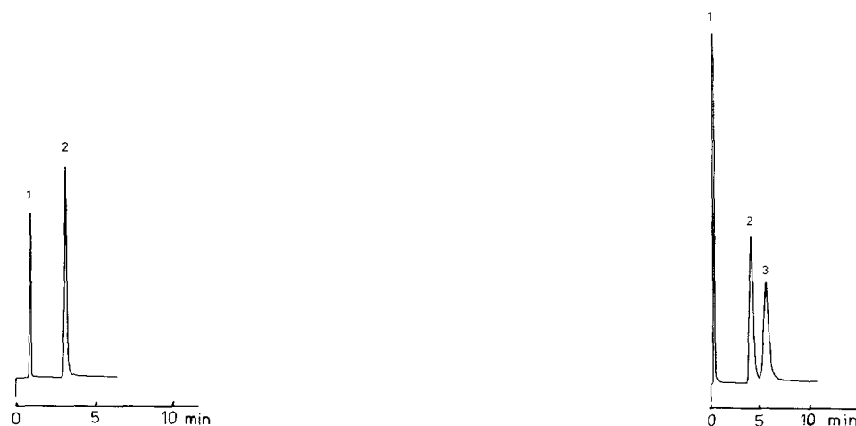
Fig. 4. Separation on a column, 20 \times 0.2 \text{ cm} I.D., packed with silica gel, modified with pyridine in plasma, \tau = 25 \text{ s} , d_p = 63\text{--}71 \mu\text{m} , temperature 90^\circ\text{C} . Peaks: 1 = Cyclohexane (b.p. 80.7^\circ\text{C} ); 2 = benzene (b.p. 80.1^\circ\text{C} ).
