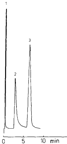
Fig. 6. Separation on a column, 20 \times 0.2 cm I.D., packed with silica gel ( 63\text{--}71 \mu\text{m} ), modified with pyridine in plasma, \tau = 25 s, at 150^\circ\text{C} . Peaks: 1 = Cyclohexane (b.p. 80.7^\circ\text{C} ; \mu = 0 D); 2 = ethanol (b.p. 78.4^\circ\text{C} ; \mu = 1.68 D); 3 = ethyl acetate (b.p. 77.2^\circ\text{C} ; \mu = 1.81 D).
